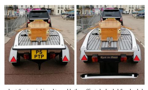
The gunwale at the stern is hinged to enable the coffin to be loaded & unloaded with ease
